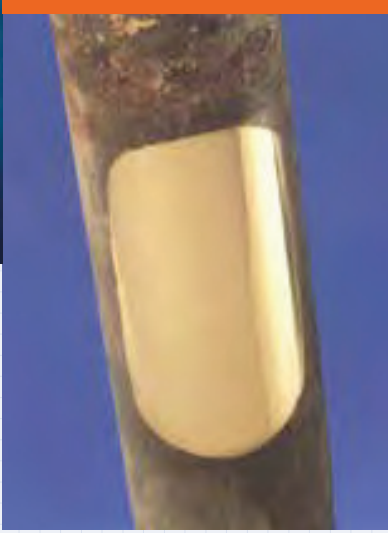
The image is an example of Tungum Tubing after 10 years at sea on a dredger. Only the grime and oxide coating has been removed from the tube exterior.
